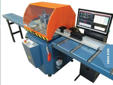
This precision semi-automatic programmable sawing system automatically rotates to cut any angle, pushes material into the saw, then automatically rotates to the next desired angle.
